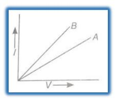
Ans: - A is series and B is in parallel, R = slope of V-I graph.
